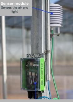
Communication module Manages power conversion & transmits data to Coretex
